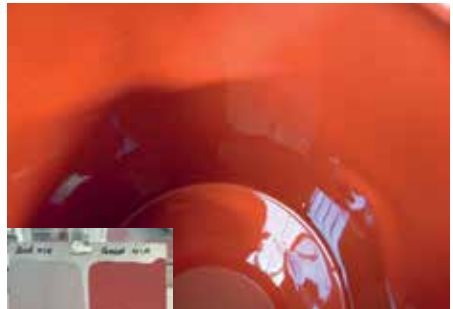
TAPOX not well enough mixed clear repellent left side.
